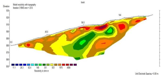
**Figure 4.** Electrical resistivity tomography at line A.
