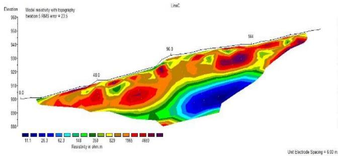
**Figure 5.** Electrical resistivity tomography at line C.
