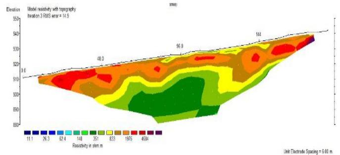
**Figure 5.** Electrical resistivity tomography at line B.
