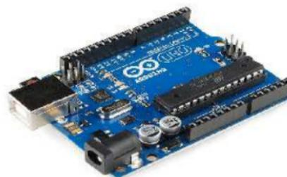
Gambar 3. Arduino Uno R3 Atmega 328
